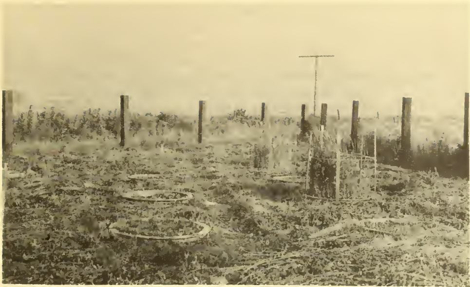
Figure 1. Evapo-transpiration tanks at Kootenai Experiment Station, Bonners Ferry, Idaho. Alfalfa has been harvested from several tanks.
