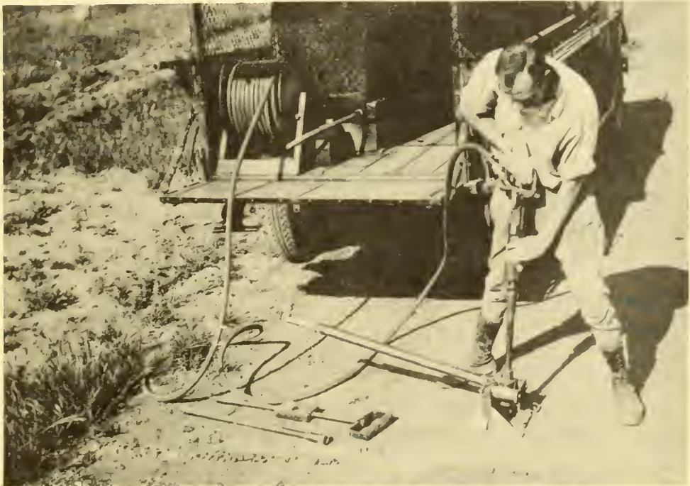
Figure 2.- Soil-sampling equipment, consisting of a soil tube, hand hammer, light air-hammer, soil-tube jack and compressor unit.
